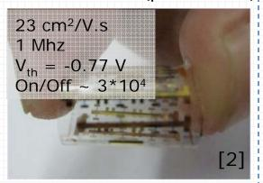
Novel approach to electronic circuits. Woven electrochemical transistors on silk fibers
